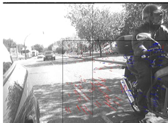
Figure 3. Optical flow results. The flow vectors appearing on the infrastructure are created by the host vehicle's ego-motion and the flow vectors appearing on the motorbike are created by the object overtaking the host vehicle.
