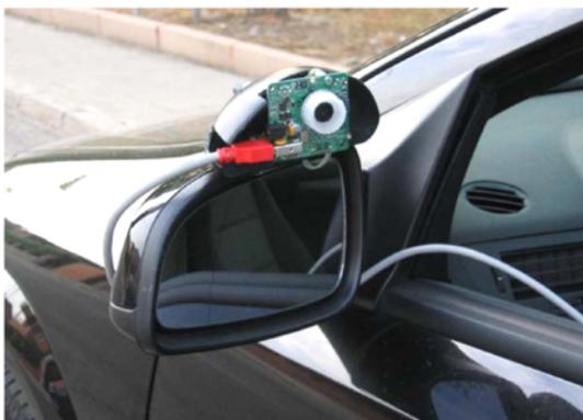
Figure 1. Side mirror prototype camera used in the experiments.
