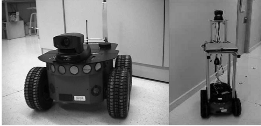
Fig. 2. Real robots Pioneer 2AT where the automatic training method has been tested.
