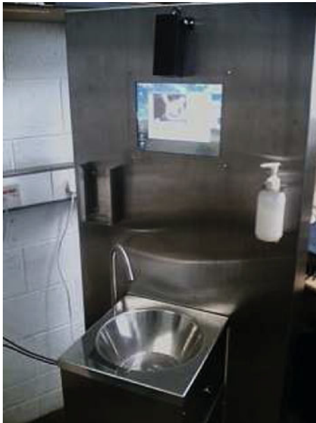
Fig. 12 Field test unit. The hand wash station uses the camera (black object) to measure the quality of the hand wash and results are displayed on the touch screen
