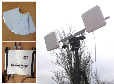
Fig. 9. Left: RFID TAGs and reader; Right: platform with RFID antennas and cameras.
