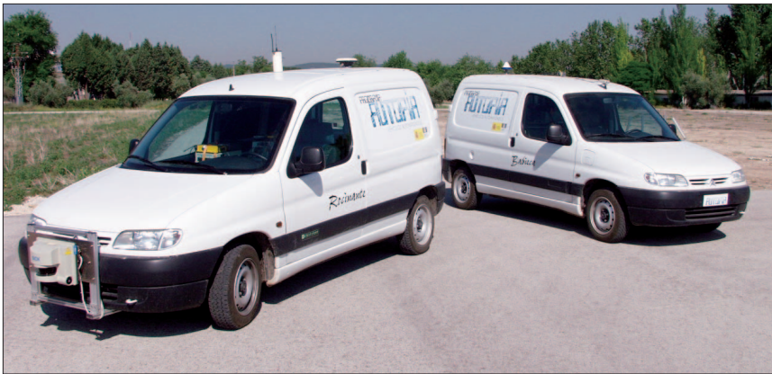
Figure 1. The AUTOPIA testbed vehicles. An embedded fuzzy-logic-based control system controls both speed and steering in each Citroën Berlingo.
