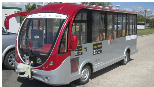
Figure 1. The drive-by-wire electric vehicle used in this experiment has capacity for 14 people. It is equipped with GPS and a multi-beam LIDAR for localization and environment recognition respectively.
