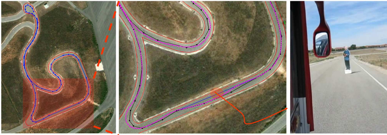
Figure 7. Trajectory is composed by a list of latitude and longitude coordinates points and speed. The autonomous mini-bus drives to the desired position at a pre-defined speed. When the destination is reached, a new waypoint is sent to the controller module. The obstacle used was a fixed dummy.
