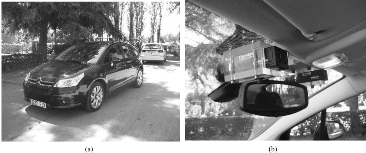
Fig. 6. (a) Prototype vehicle, (b) stereo-camera platform on-board the vehicle.
